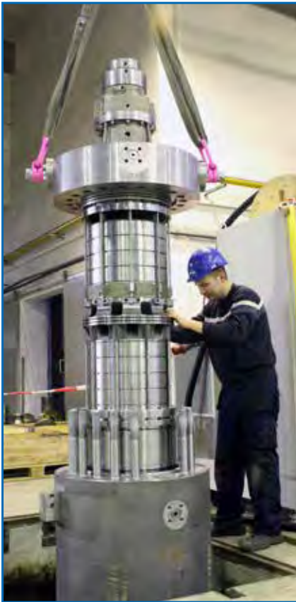
■ Assembly of an insert unit for horizontal process barrel pump.
