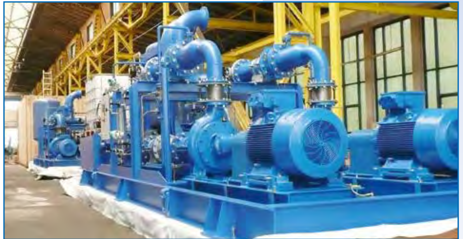
▪ Transfer Pump Skid
